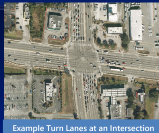
Example Turn Lanes at an Intersection
