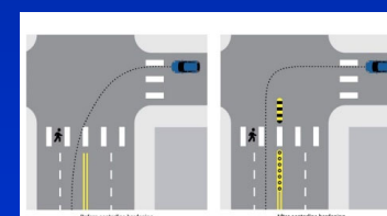
Hardened Centerlines/Pedestrian Refuge
